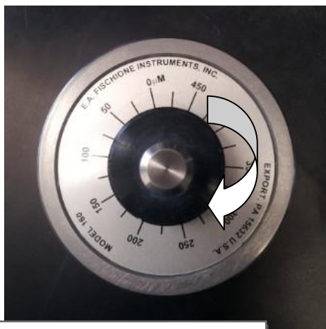
Puck thickness control. Turn clockwise to lower sample toward polishing wheel
