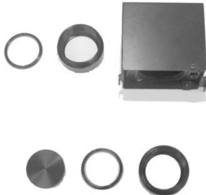
(In this image, the dummy filter is at the bottom left.)
