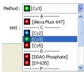
From the pull-down menu, select the method that corresponds with the sample. The selected laser and filter combination is displayed on the right.
