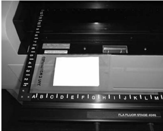
**Note:** To reduce the effect of physical vibrations place a membrane weight on top of the **membrane samples**.
