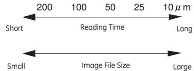
The 10  $\mu\text{m}$ -pixel size processing is conducted by applying Bi-cubic algorithm to the images read at 25  $\mu\text{m}$ -pixel size. Therefore, computer processing after reading may take a longer time than image reading time.
