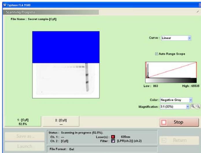
**Note:** If you click the **Stop** button during reading, the part that has not been read yet will be saved as an image with a data value of 0 (light intensity of 0).
