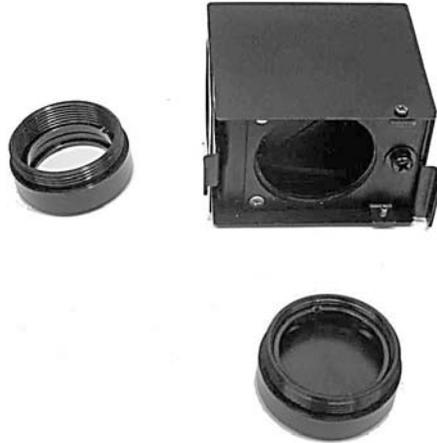
(In this image, the lower filter holder contains a dummy filter.)
